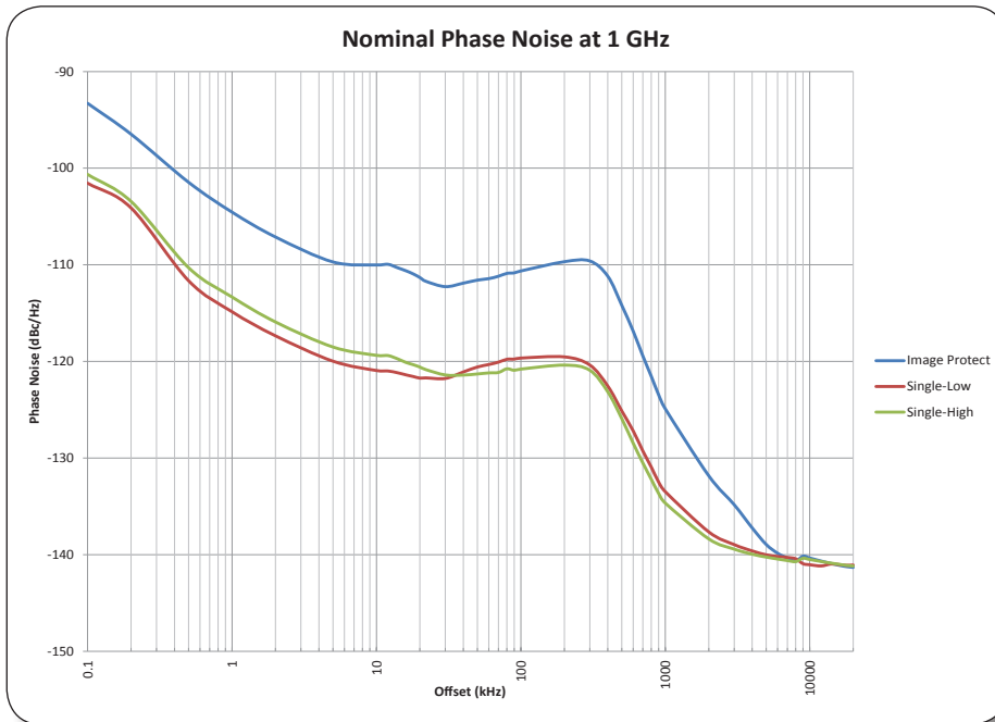
Figure 8. Phase noise at 1 GHz (1.1 GHz for single-low conversion type).
